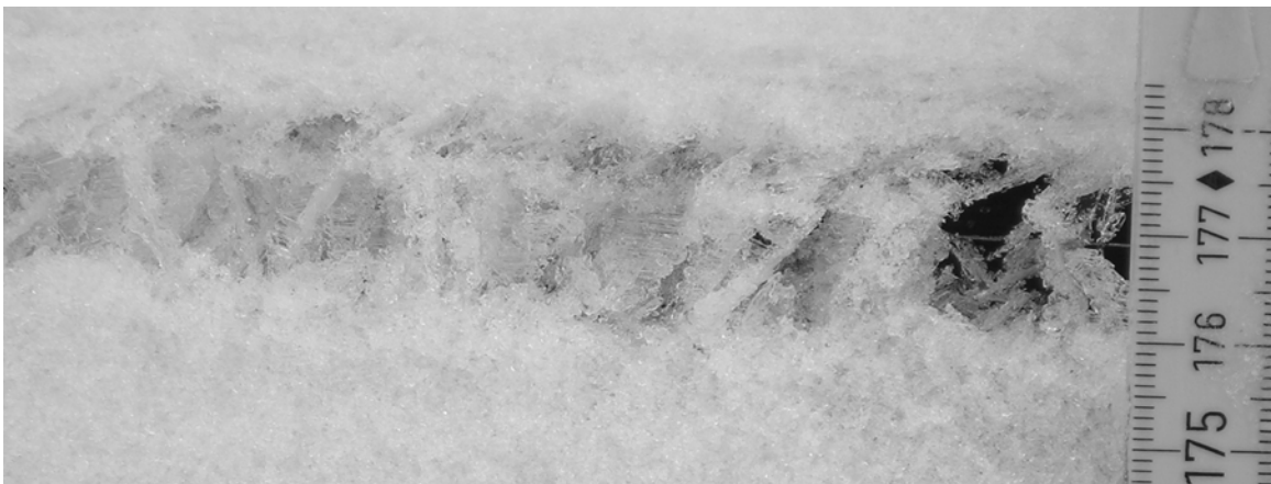
Figure 48. Close up photo of the double surface hoar layers. Ruler marked in centimeters.
