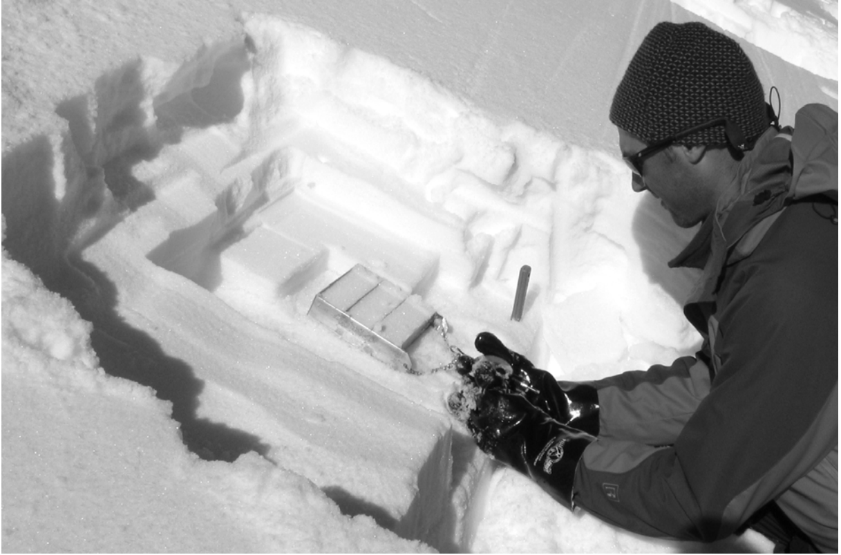
Figure 11. Kalle Kronholm conducting a shear frame test. The frame has just failed, and the force at failure is being read.
