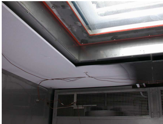
Figure 19. Longwave simulation panel mounted on the chamber's ceiling. Note the condensation on the ceiling panel. The solar lamp is shown in the upper right.
