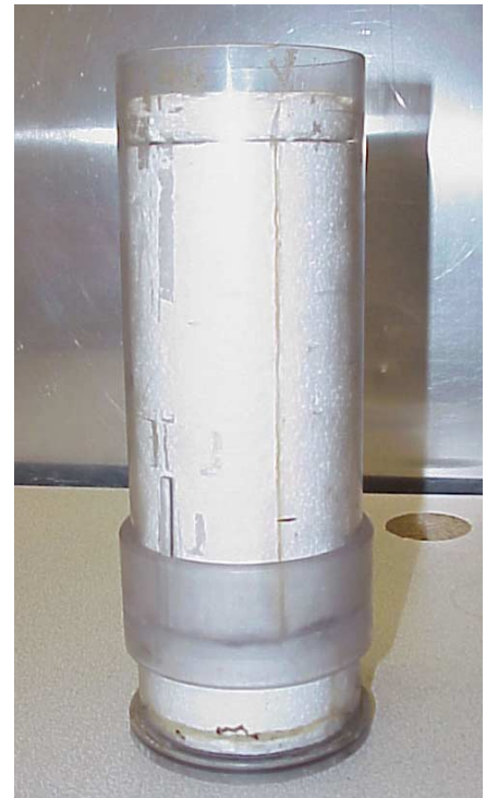
Figure 14. Chamber for keeping snow samples frozen during CT scanning.
