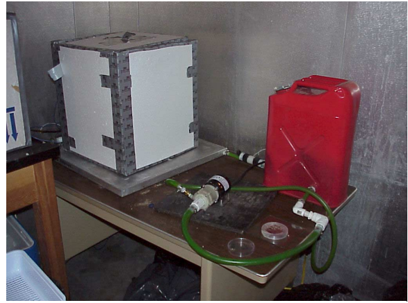
Figure 13. Experiment configuration showing styrofoam box, aluminum temperature plate, and heating system.
