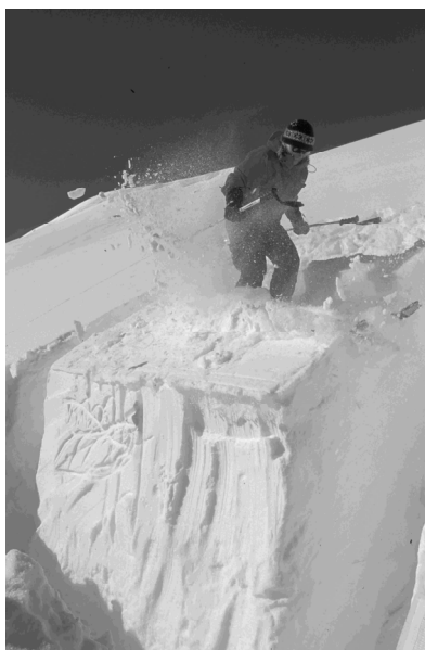
Figure 2.16. The rutschblock during loading in step 4; jump from above the block with skis.
