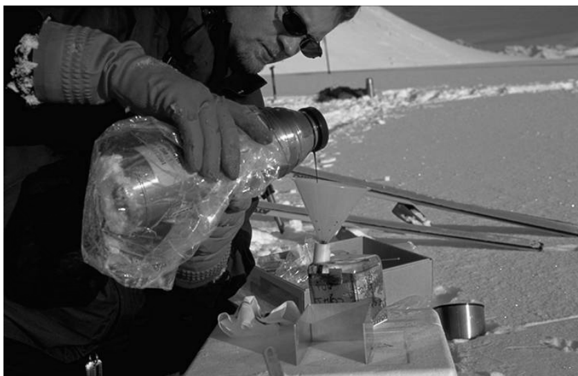
Figure 2.10. After removal of the sample from the wall of the snow pit, black diethyl-phthalate was slowly poured into the sample until it was completely saturated.
