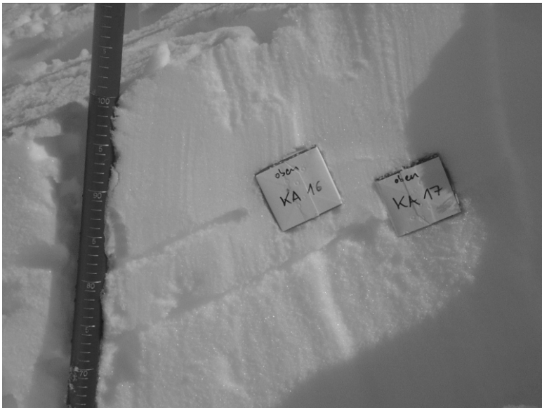
Figure 2.9. Two in-situ samples were taken parallel to the snow layers on the vertical wall of the snow pit in grid 20. Removal of weak layer samples from the wall often had to be repeated several times to get an undisturbed sample.
