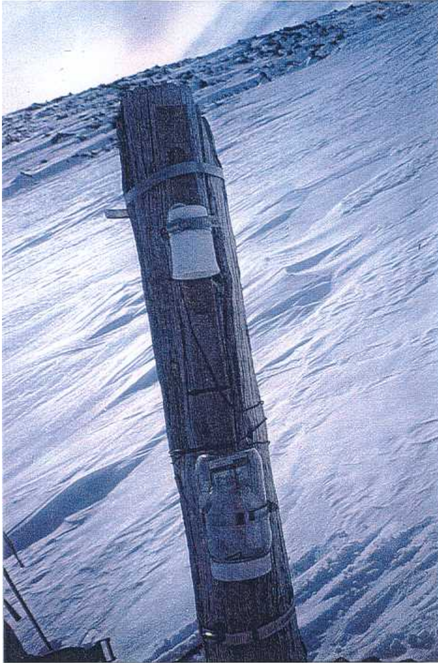
Figure 4.2: Field setup of Hobo data logger and air temperature sensor. The temperature sensor is placed in an inverted plastic cup that serves as a radiation and precipitation shield. The data logger is located in a plastic jar below the radiation shield.
