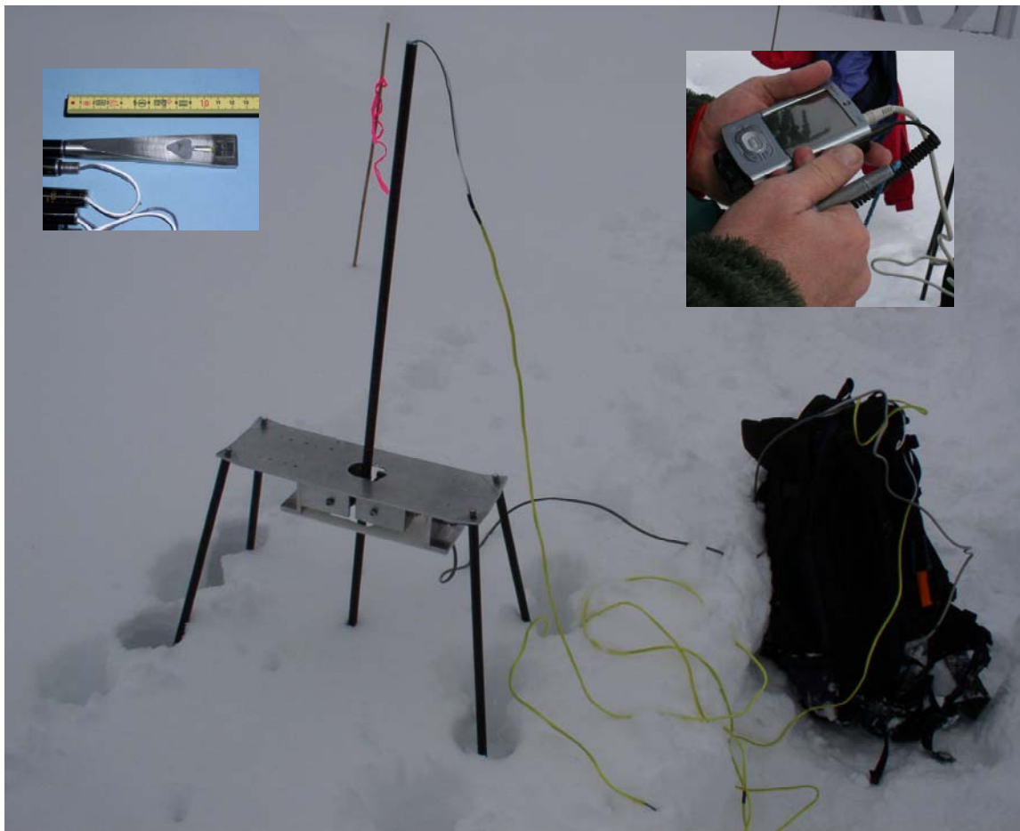
Figure 4. Illustration of second-generation probe following a full depth plunge, encoder, and backpack containing electronics. Upper right insert shows the PDA and A-D device, upper left insert shows the probe tip and collapsed avalanche probe shaft.
