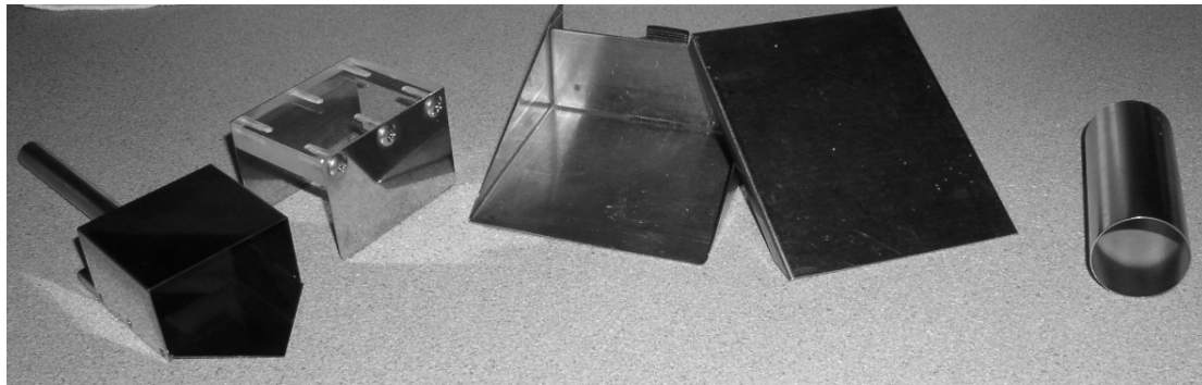
Figure 7. Various types of density cutters tested for variance, left to right: box (100 cc), wedge (200 cc), and tube (100 cc).
