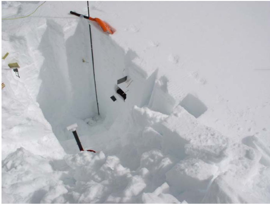
Figure 6. Typical data collection excavation showing the probe as left in place for vertical measurement reference following final plunge of day's sequence. Manual densities were measured directly adjacent to probe.
