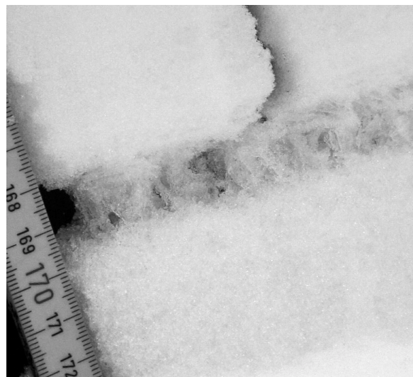
Figure 2: The Montana weak layer consisted of two layers of surface hoar stacked on top of one another. The slope collapsed on the upper of the two layers. This photo was taken at the tensile fracture, showing the collapsed layer (left of the fracture) and the uncollapsed layer (right of the fracture). Ruler is marked in cm. Photo by E. Lutz.
