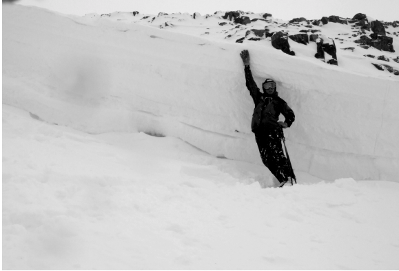
Figure 7: The Big Sky avalanche. A tensile crack opened up when the slope was tested with the first 1 kg shot. Noting the crack, the control team applied a second 1 kg shot and released this avalanche. The HS-AE-R3-D3 slide released 1.2 to 2.1 m (4 to 7 ft) deep on faceted snow overlying a crust.
