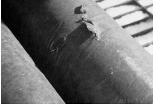
Figure 9: Shrapnel embedded in a cardboard storage tube containing a live 106mm RR round. The tube was lying on the mount.
