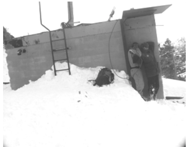
Figure 11: 106 mm RR Mammoth Mountain Gun Mount after in-bore explosion. Note weapon lying in the snow in front of the mount.
