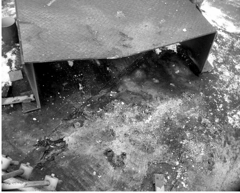
Figure 13: Severe damage to the protective box that contained live rounds when the in-bore explosion occurred.
