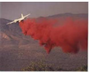
Fatal mishap: Airtanker was in 60 degrees of bank turning towards the drop site. The bank suddenly increased to 90 degrees and the aircraft struck the ground. High winds and turbulence reported in the area.
