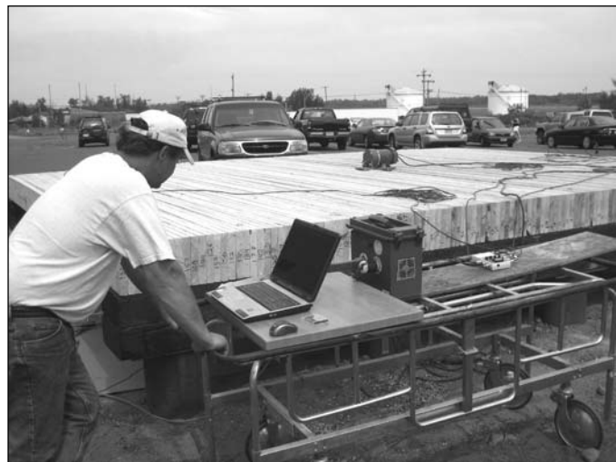
Researchers conducting forced vibration testing.
