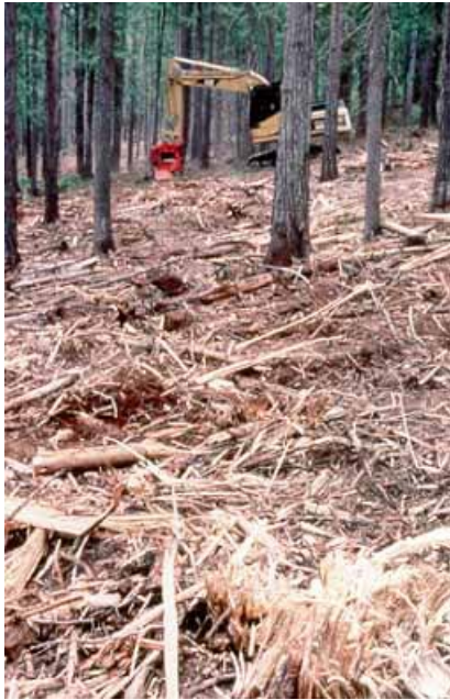
The Slashbuster breaks up forest thinnings and scatters them on the forest floor. FPL researchers are studying what affect this and other treatment techniques have on forest health and the risk of wildfires.
