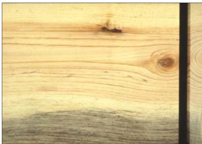
The bluish-black discoloration is blue stain. Note that the stain penetrated through the sapwood of this crosscut specimen.
