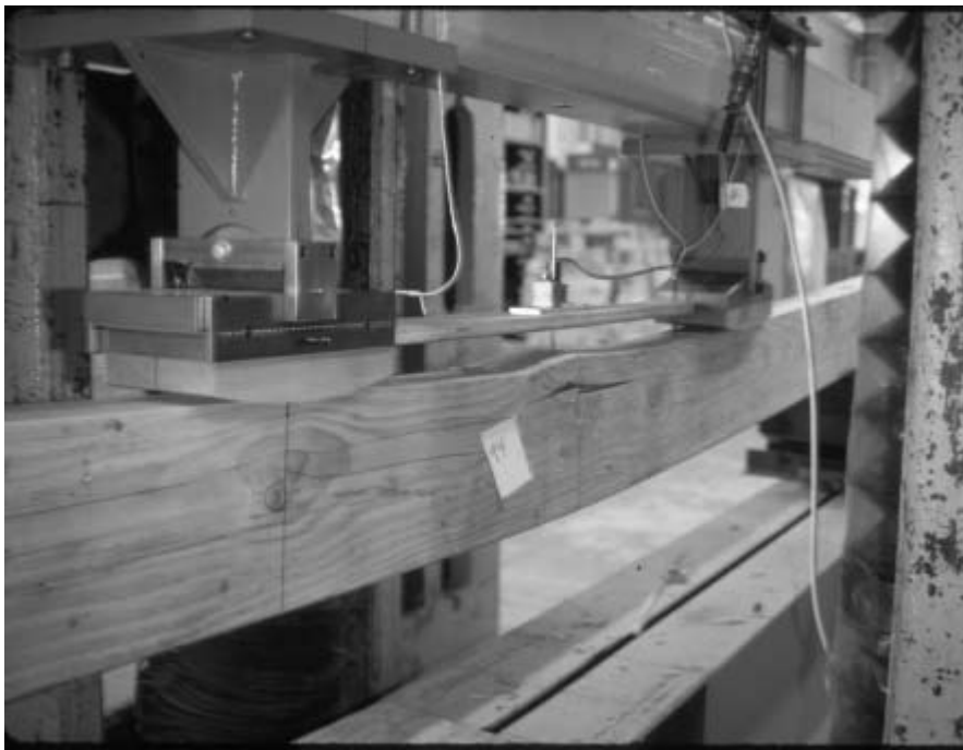
Figure 8. — Local buckling around hole in group A beam.
