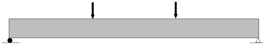
Figure 3. — Test configuration and hole layout for group C (control) beams.
