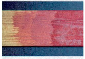
Too many coats have the opposite effect. More than one coat of semitransparent oil-based stain can be applied as long as subsequent coats are applied while the first is still wet and as long as not so much is applied that a film forms on the surface.
