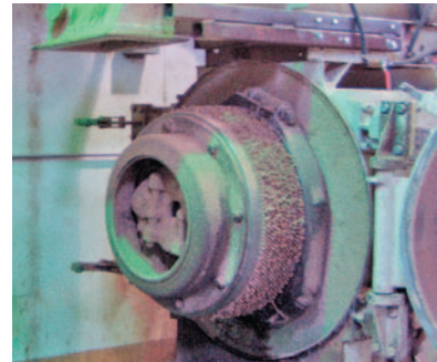
Pellet Mill with cover open
