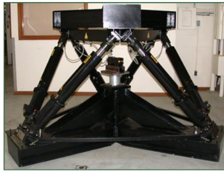
Six-axis test machine developed at FPL for evaluation of multi-axis strain-stress relations.
