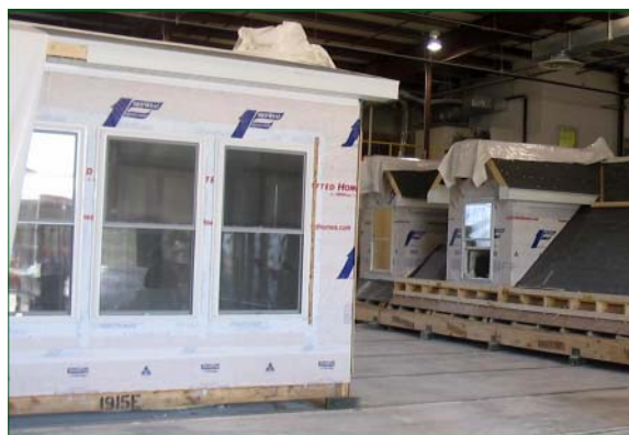
Two modules near completion as they progress along the manufacturing line in a modular home factory.
