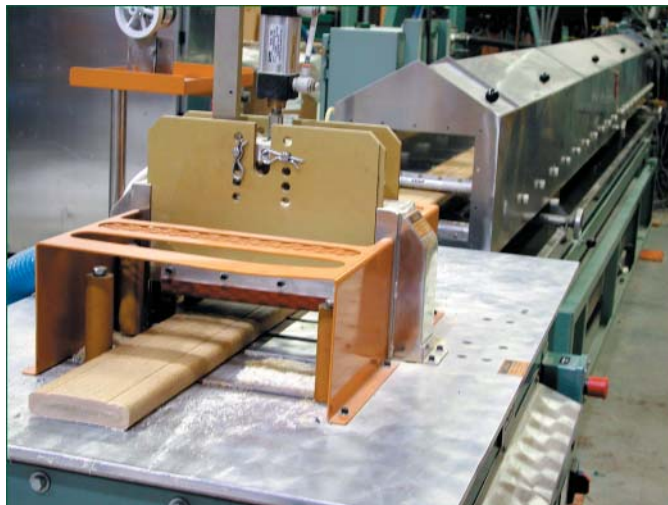
Extrusion of WPC lumber at the University of Maine.
