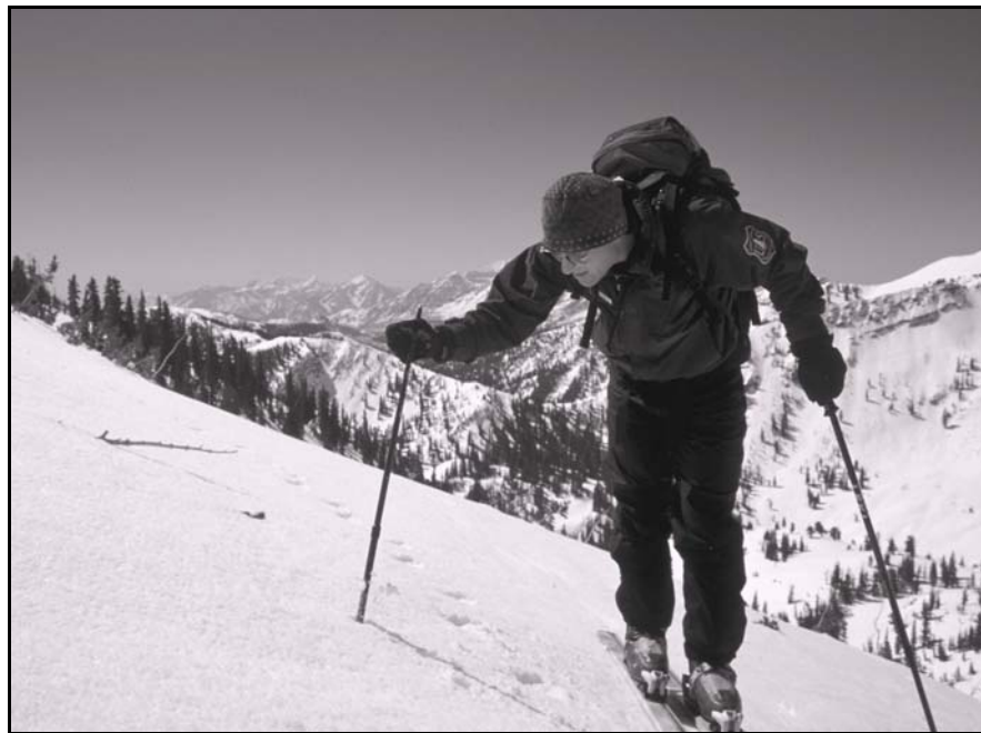
Figure 2.20 The ski pole poke, aka ski pole penetrometer (photograph by Bruce Tremper).
