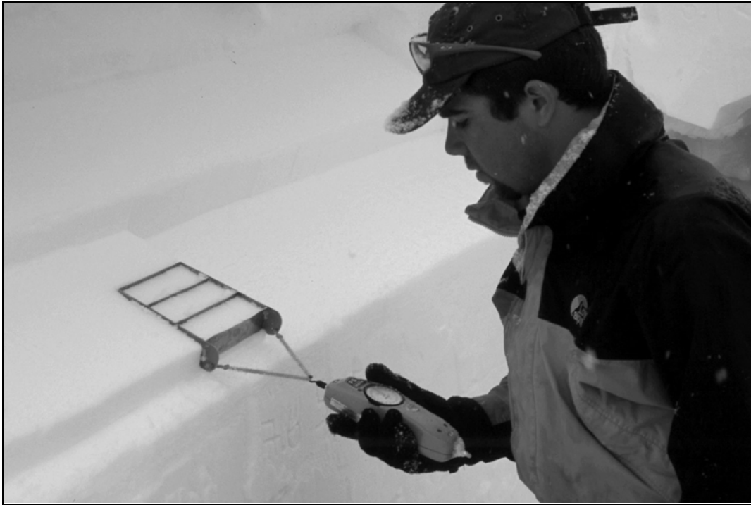
Figure 2.25 Measuring the shear strength of a surface hoar layer with a 250 cm 2 shear frame and force gauge (photograph by Greg Johnson).
