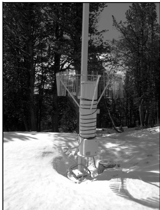
Figure 1.5 Precipitation gauge with Alter shield (photograph by Tom Leonard).
