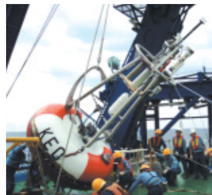
The moored buoy in the Kuroshio current in the north Pacific returned 100 percent of surface data. Measurements from the Kuroshio Extension Observatory will contribute to climate studies of the role of the Kuroshio jet and its recirculation gyre. Photo: Japan Agency for Marine Earth Sciences and Technology
