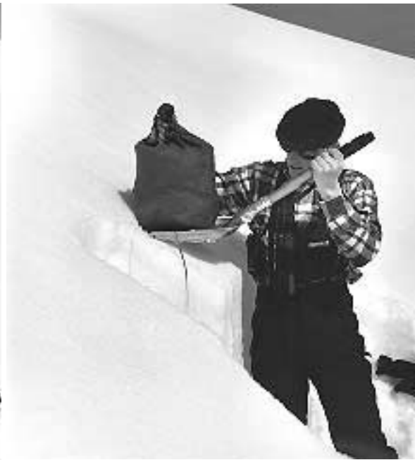
Figure 4--The sack is gently placed on top of the isolated column of snow.
