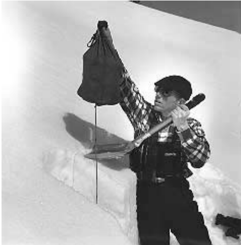
Figure 5a--If the column does not fail when the sack is gently placed on top of the isolated column, the block is loaded dynamically. The stuff sack is lifted in increments of 100 mm (4 in) . . .
