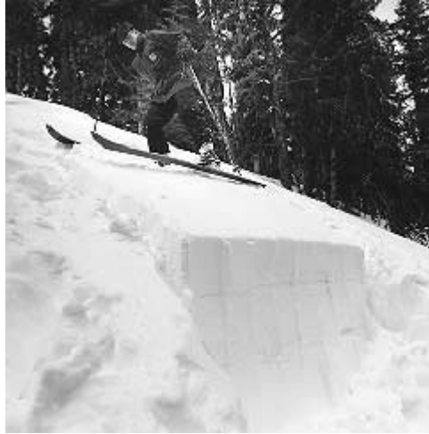
Figure 8--If the rutschblock does not fail when it is isolated, it is progressively loaded by a person on skis. First, the person gently steps onto the block. A failure at this point would indicate a rutschblock score of 2.
