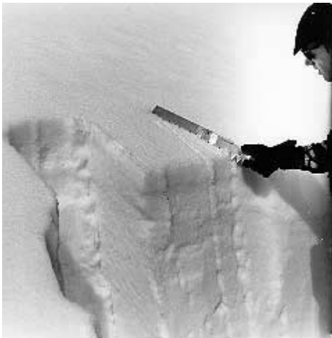
Figure 2a--A block of snow 300 mm (12 in) square is isolated from the snow pit wall by cutting out the sides.
