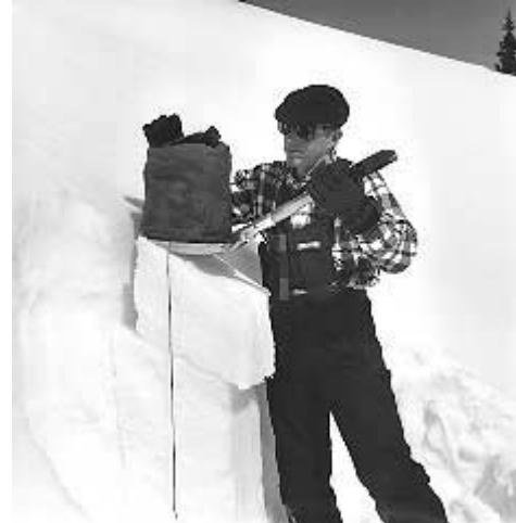
Figure 5b-- . . .and dropped onto the column until it fails.
