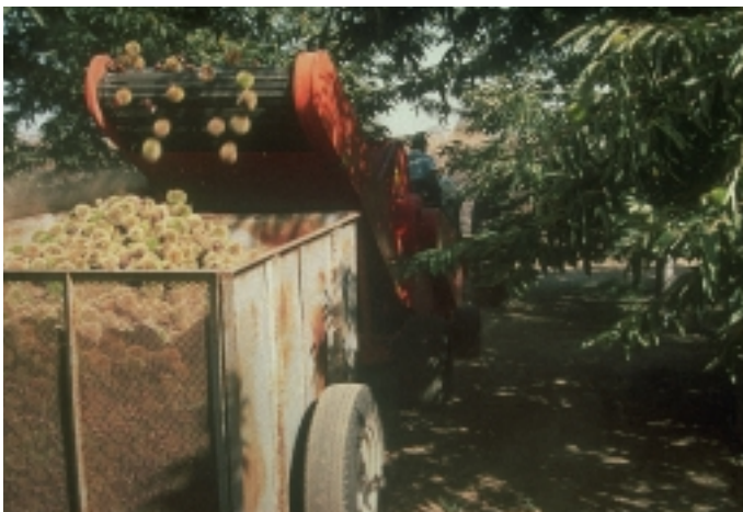
Figure 15. A conveyor belt from a pick-up machine loads chestnuts into a bin.
