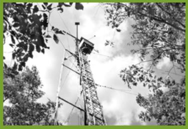
One of the eddy flux towers at Silas Little Experimental Forest in the New Jersey Pine Barrens. Measurements of energy, water vapor and net CO. exchange started in April 2004. Annual net CO<sub>2</sub> exchange (NEEyr) measured at this site ranges between 187 and -293 g of carbon per m<sup>2</sup> per year, with the largest carbon loss value corresponding with complete defoliation by the gypsy moth in 2007.
