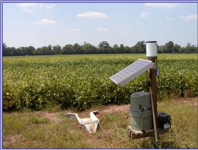
Automatic water samplers were installed at each of the sites.
