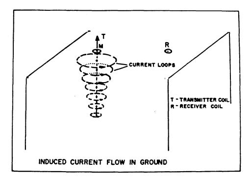
Figure 8. Diagram showing the principle of operation of electromagnetic induction soil conductivity sensor.
