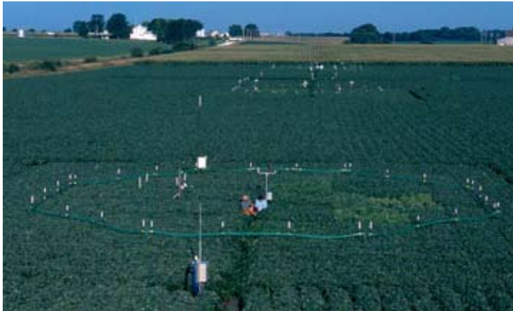
Scientists Carl Bernacchi, ISWS, and Bruce Kimball, U.S. Arid-Land Agricultural Research Center, Maricopa, Arizona, measure photosynthesis and water use of soybeans grown in elevated CO 2 at the SoyFACE research facility in Champaign.
