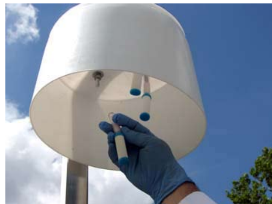
Triplicate sets of passive diffusion sampling tubes mounted in a simple shelter measure ammonia gas concentrations at remote monitoring sites. These comparatively inexpensive devices require no electricity and are not subject to breakage during handling and shipping. Exposure times of two weeks or less are sufficient for part-per-billion ammonia quantitation.
