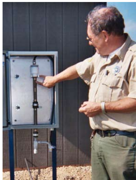
A much simpler ISWS shop-built sampling system extracts ammonia and related acidic gases from air drawn at controlled flow rates through specially designed gas denuders. After each 24-hour sampling period, field site operators manually remove, pack, and ship exposed denuders for laboratory analyses.
