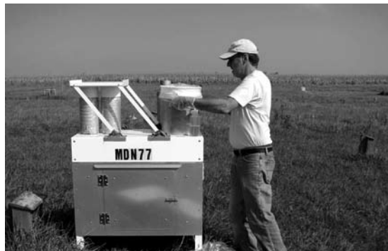
Bondville site operator Mike Snider regularly collects samples from equipment that measures mercury.
