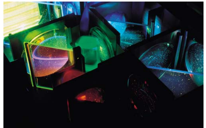
Magnified view of Philips' color optics. Mirrors separate and recombine the red, green, and blue colors.
