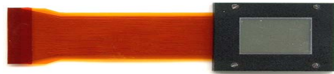
Example of a Kopin CyberDisplay LCD, with 0.25-inch diameter, used for a microdisplay.
