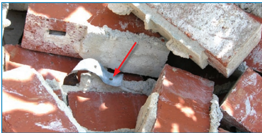
Figure 3-46: This tie remained embedded in the mortar joint while the smooth-shank nail pulled from the stud.
