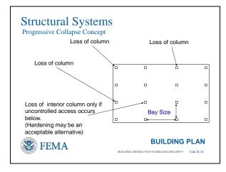
NOTE: The BAY SIZE is the distance between columns in the vertical and horizontal directions. The Bay Size can be identical or different in any part of the building and change between different parts of the building.
