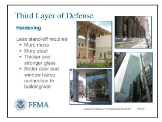
U.S. Embassy: Kampala, Uganda designed to resist explosive blast [upper left – DOS and Hinman]. Other three photos are from New York City indicating glass and overhang (poor) [lower left], similar glass and overhang (poor) but with wall (better) [upper right], and window curtain wall (usually poor) [lower right].
