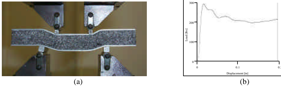
Figure 1. Flexural testing (a) deformed geometry (b) typical load-displacement curve.
