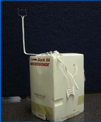
Radiosonde used by the RRS
