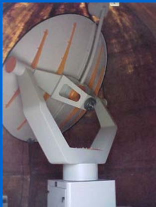
Tracking antenna for the Radiosonde Replacement System (RRS)
