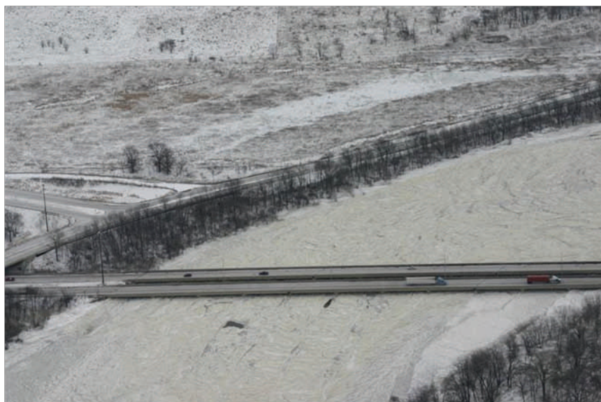
Ice jam on the Kankakee River at the I-55 Bridge near Wilmington, IL.
