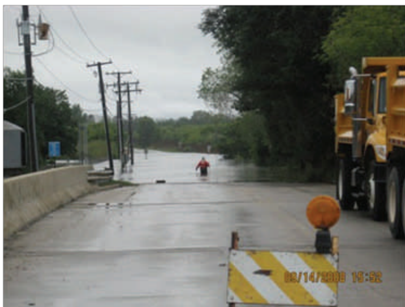
USGS Hydrologist David Schrader makes a wading road overflow measurement at the USGS gage at On the East Branch Du Page River in Bolingbrook, IL
