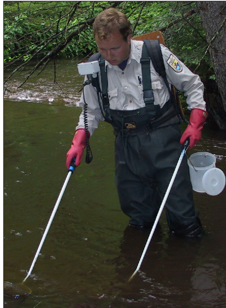
Electroshocking is an efficient way to measure fish abundance for some freshwater species.
