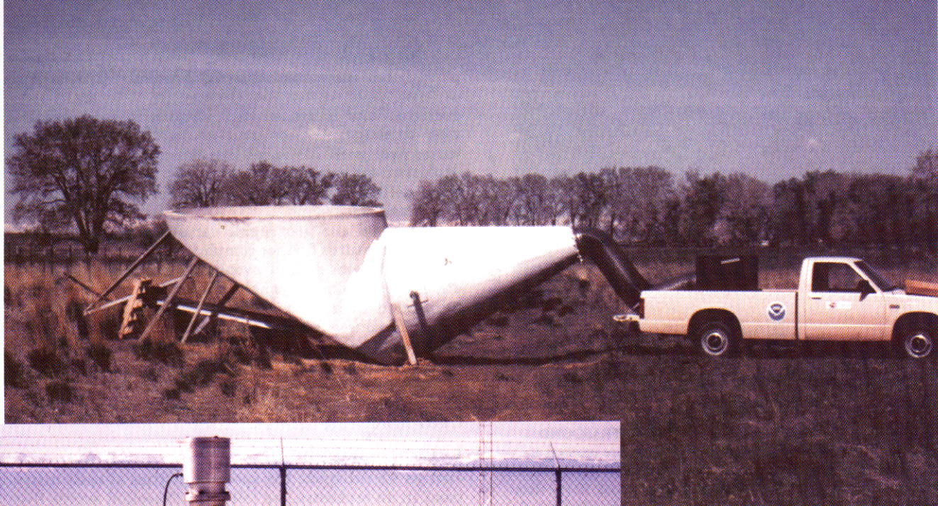
FIGURE 1. EXPERIMENTAL LOW-FREQUENCY SOUND GENERATORS are used for remote probing and propagation studies. The 10-foot-diameter horn (above) produced audible sound at 100 Hz, which was tracked with a Doppler radar to altitudes of 20 kilometers to obtain temperature profiles of the atmosphere. The 100-gallon sphere with a 1 m neck (left) is a Helmholtz resonator tunable from 10 to 50 Hz. Compressed air is released by rupturing a diaphragm, producing sound waves used for calibrating and testing infrasonic arrays.
