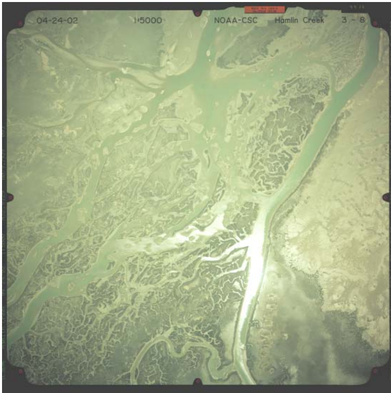
Figure 4. Conventional color aerial photograph of the Hamlin Creek area. Scale is 1:5,000. This photography has high spatial resolution but limited spectral information to guide automated processes.
