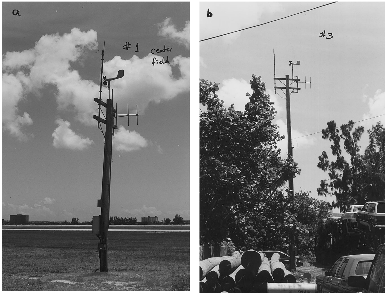
FIG. 7. Examples of contrasting exposures for LLWAS sites FA1 (a) and FA3 (b) plotted in Fig. 6.
