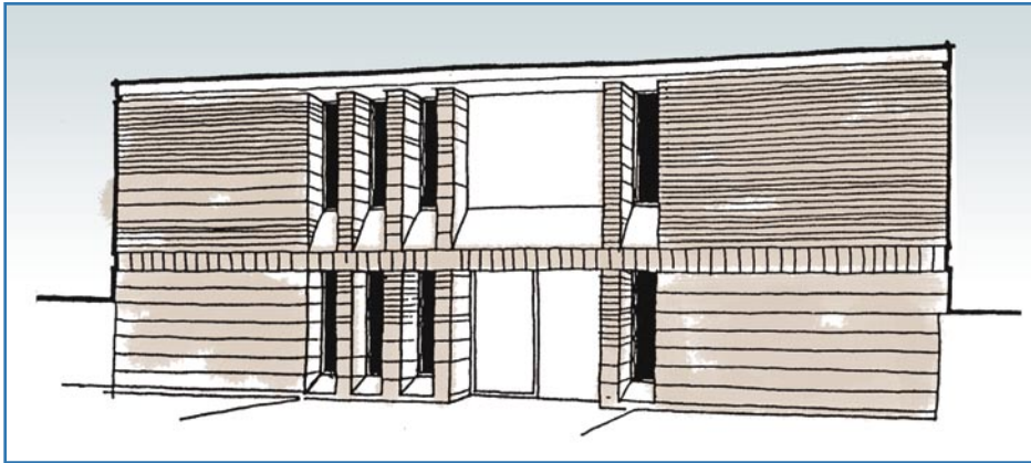
Figure 3-6 Narrow and recessed windows with sloped sills
