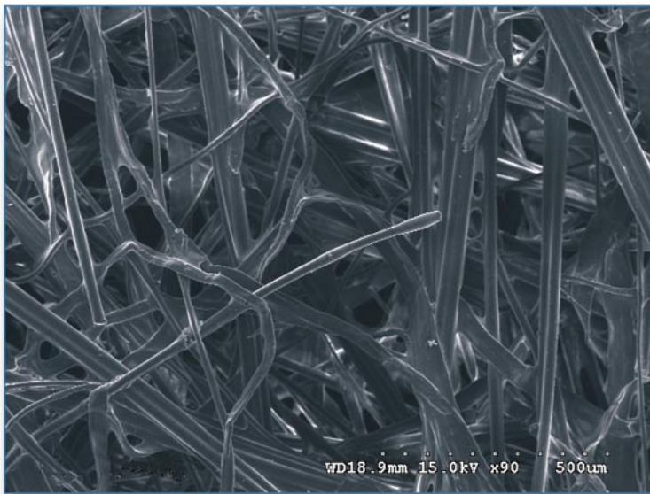
Figure 5-2 Scanning electron microscope image of a polyester-glass fiber filter
