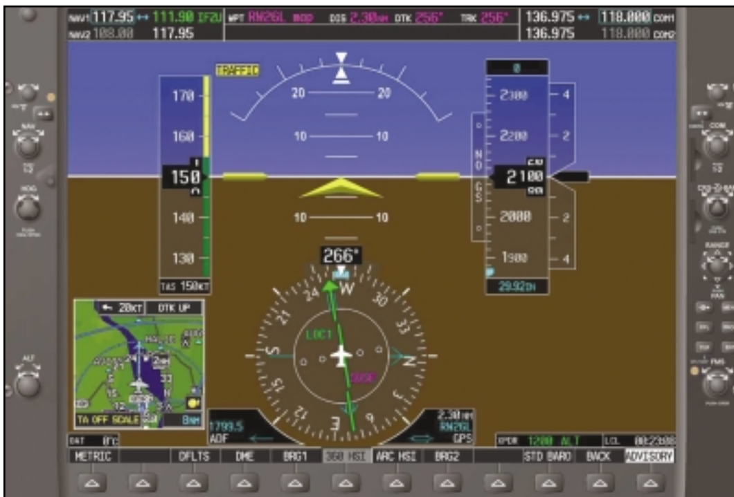
The G1000® Primary Flight Display (PFD) offers the pilot communications, navigation, and aircraft flight information as well as pilot selectable options such as the insert map.
