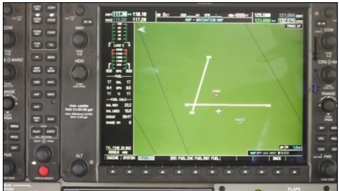
The Garmin G1000® Multi-Function Display can display runway information as part of its navigation displays. Airport frequencies, layout, and other data are readily available.
