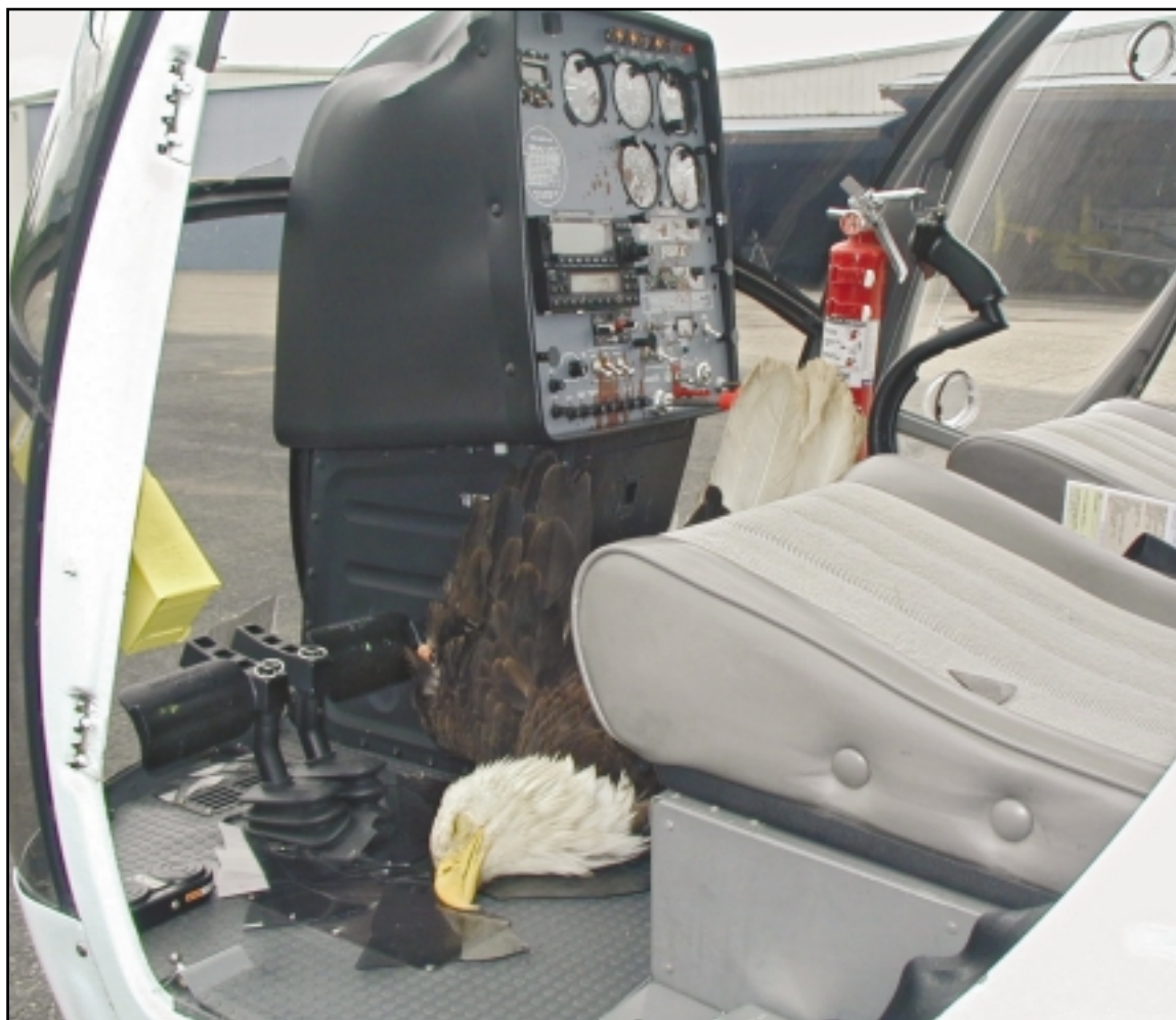
This eagle hit the helicopter's passenger causing several injuries to her chest, face, and fracturing her shoulder. The strike occurred at 2,000 ft. AGL over Eden Prairie, MN. Aircraft repairs cost $10,000. (photo by Chris Cooper, Hummingbird Helicopters)
