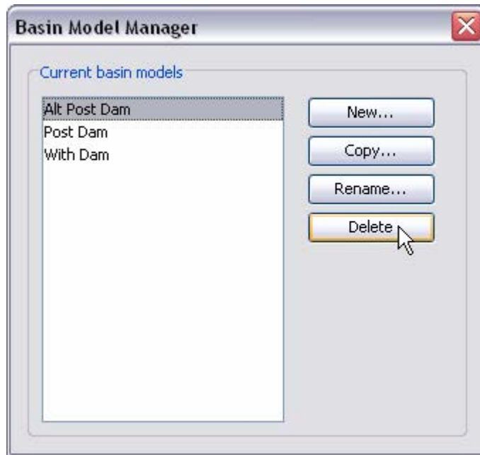
Figure 76. Preparing to delete a basin model from the Basin Model Manager. A confirmation will be required after pressing the Delete button.
