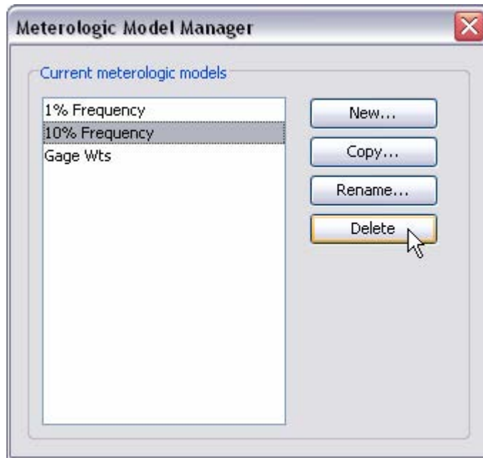
Figure 144. Preparing to delete a meteorologic model from the Meteorologic Model Manager. A confirmation will be required after pressing the Delete button.
