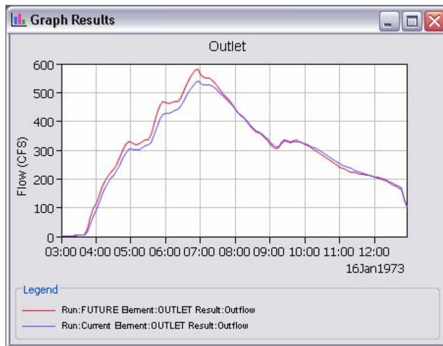
Figure 193. Custom graph created by selecting multiple time-series results for a preview and then pressing the graph button on the toolbar.
