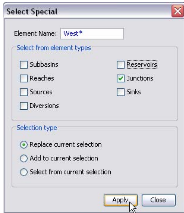
Figure 92. Using the special selection tool to select all junctions whose names begins with the letters "West".
