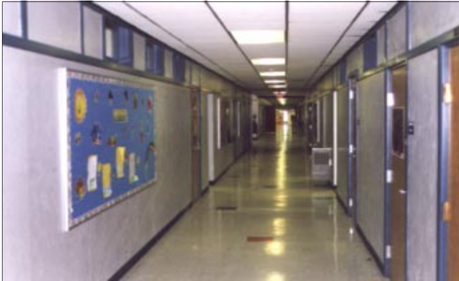
FIGURE 6-33: Sooner Rose Elementary School, Mid West City, Oklahoma. According to the tornado plan for this school, this hallway is designated as a place of refuge – double loaded corridor.
