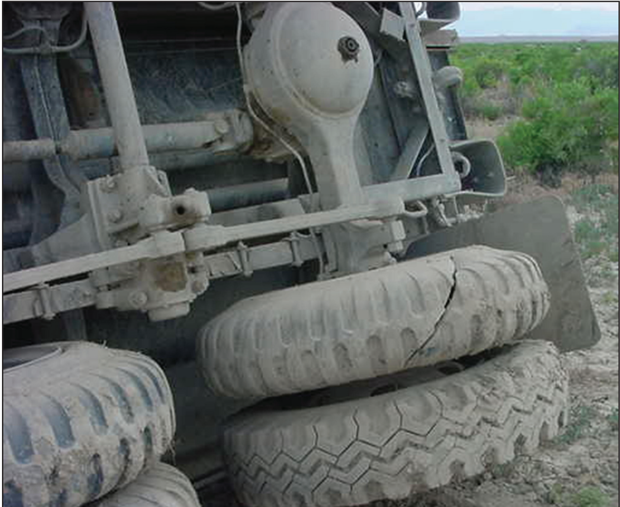
Photo 5. Interior tire on the back rear axle of the passenger's side Photo courtesy of the State forestry department
