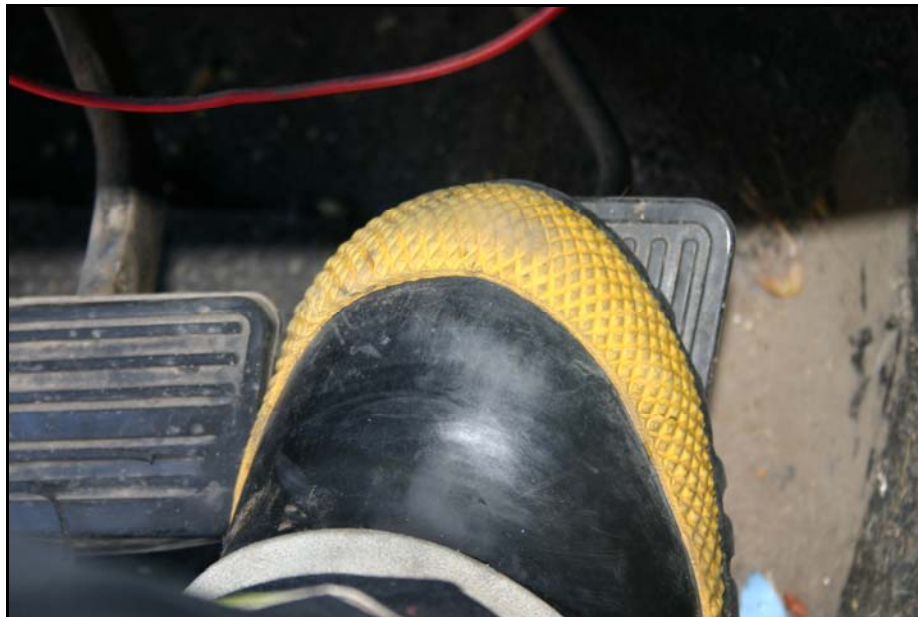
Photo 5. Rubber fire boot caught between pedals and comparison of boot size to pickup truck's pedals.
