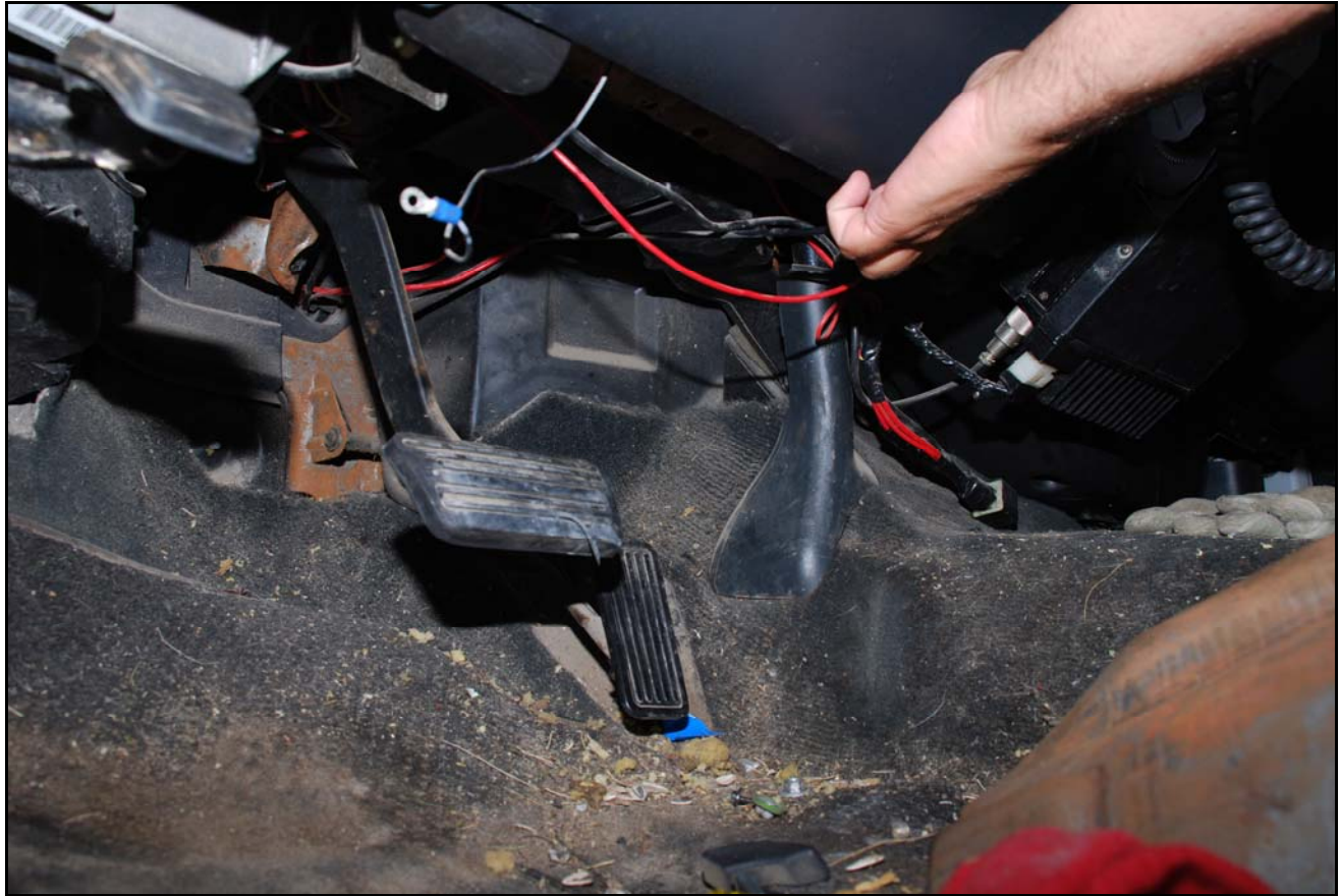
Photo 6. Hand pressure being applied to exposed siren cable causing accelerator pedal to go to floor. (Photo courtesy of Sheriff's Office)
