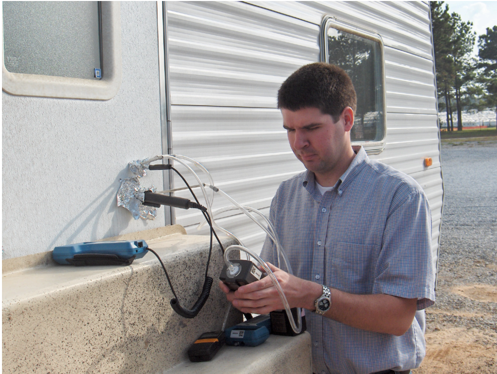
Figure 2. Collection of indoor sample through the THU door.
