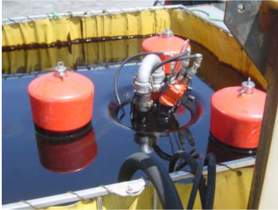
Figure 2: Weir skimmer in portable tank for control test
