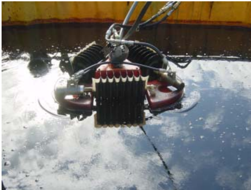
Figure 1: Disc skimmer in portable tank for control test
