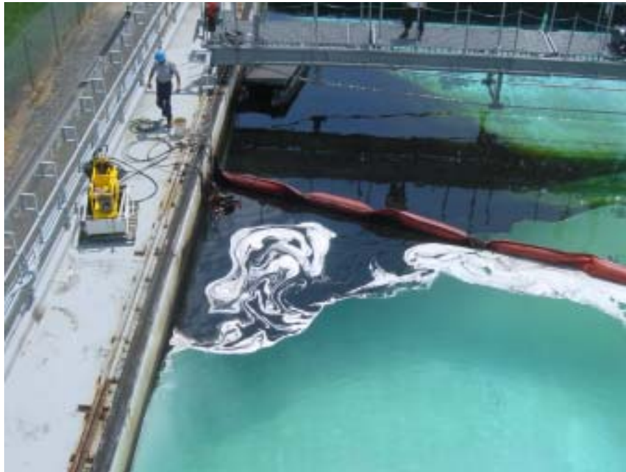
Figure 3: Oil accumulated for skimming between boom and tank wall
