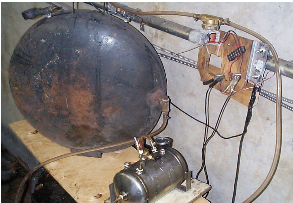
Figure 4: Dispersant Spray Pressure Tanks & Valve
