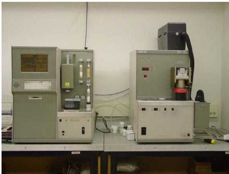
Figure 14 - LECO Hydrogen Determinator RH-404. On the left is the unit that measures that hydrogen concentration and on the right is the electrode furnace.
